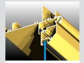
The continuous hinge built into the head and top of the sash is designed to carry heavy sashes and protect the top of the sash from water intrusion.
